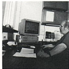
If the Meg-Alert™ unit detects an insulation weakness in one of the motor/pump units, a message comes up on the computer screen at the remote monitoring station.
